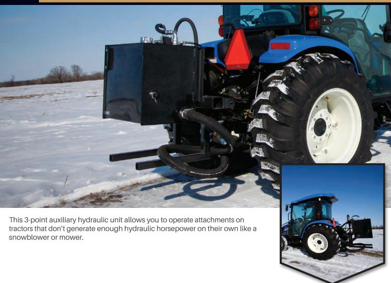
THE HYDRAULIC PUMP OFFERS SUPERIOR PERFORMANCE OVER ANY OF OUR COMPETITORS BECAUSE IT GENERATES HIGHER GALLONS PER MINUTE
