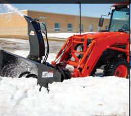
THIS SELF-CONTAINED UNIT PRODUCES **ENOUGH GALLONS PER MINUTE** ALLOWING YOU TO OPERATE THESE **HYDRAULICALLY-DRIVEN ATTACHMENTS**
