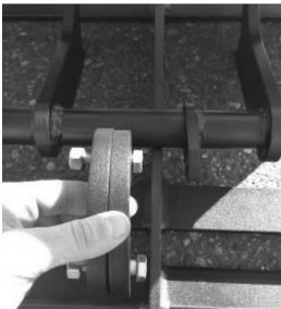
3. Loosen the (2) bolts from the pivot pins and remove the pins, replacing the bolts into the pins for future use.
