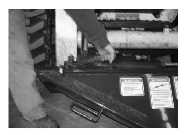
6. Secure the coupler locking mechanism that attaches the attachment to the loader.
