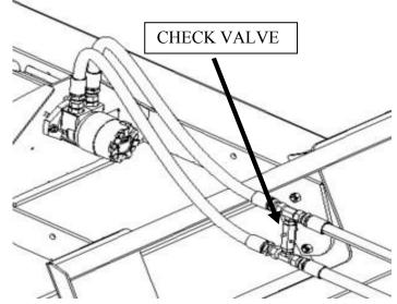
If the mower is run with the oil flow in reverse, the oil will bypass through the check valve and the mower will not operate correctly. Symptoms could include very low speed and a lack of power.
