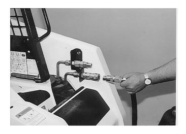
**NOTE:** Attachment is shipped with 8FJX (3/4" Female JIC Swivel) fittings on the ends of the lead hoses.
