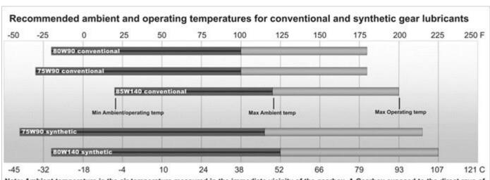
Note: Ambient temperature is the air temperature measured in the immediate vicinity of the gearbox. A Gearbox exposed to the direct rays of the sun or other radiant heat sources will operate at higher temperatures and therefore must be given special consideration. The max operating temperature must not be exceeded under any circumstances, regardless of ambient temperature.
