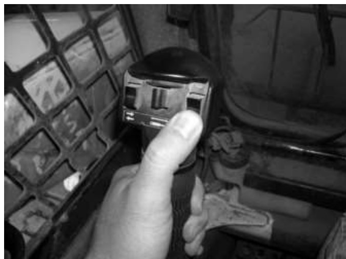
PUSH AND HOLD TO ENERGIZE DIVERTER
