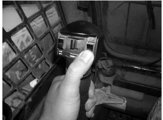
PUSH AND HOLD TO ENERGIZE DIVERTER
