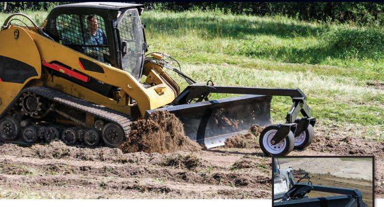
Turn your skid steer into a high performance, dirt moving machine. This dozer, grader, and leveler is an all-in-one package. Ideal for dozing, scraping, and cutting swales, as well as leveling roads, yards, and job sites. Six-way hydraulically controlled dozer blade is easy to operate. Saves job site prep time.
