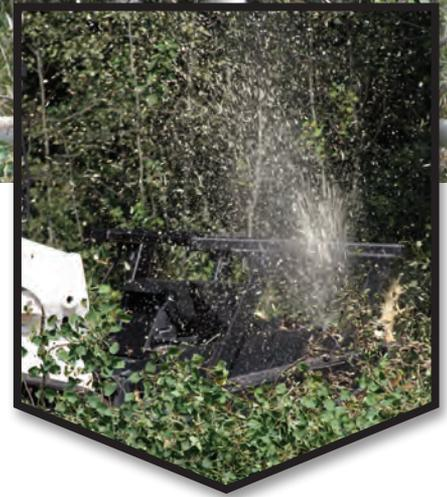
Our Forestry Mulching Mower is designed to de-forest an area and return the debris back to the environment. This Forestry Mulching Mower cuts trees up to 14" in diameter and mulches trees up to 6". If you need a powerful, reliable mulching mower in your arsenal, you need our Forestry Mulcher Mower.
