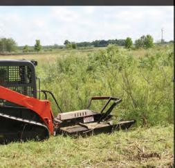
THE OPEN DECK DESIGN ALLOWS **CUTTING OF LARGER TREES**
