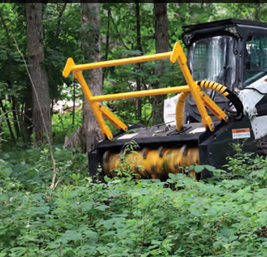
THREE POSITION ADJUSTABLE PUSH BAR FOR ALL YOUR FORESTRY APPLICATIONS
