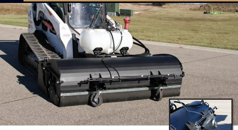
Sweep, clean and scrape mud going forward or in reverse. Ideal for construction, industrial or municipal jobs, the Heavy-Duty Pick-Up Broom is easy to attach and simple to operate on your skid steer. The reversible cutting edge helps cut loose caked-on mud, while the sweeper's poly bristles deposit dirt and debris in the container which can be dumped when full.
