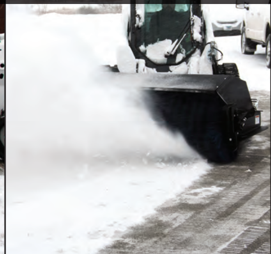
OSCILLATING DESIGN ALLOWS BROOM TO FOLLOW UNEVEN TERRAIN
