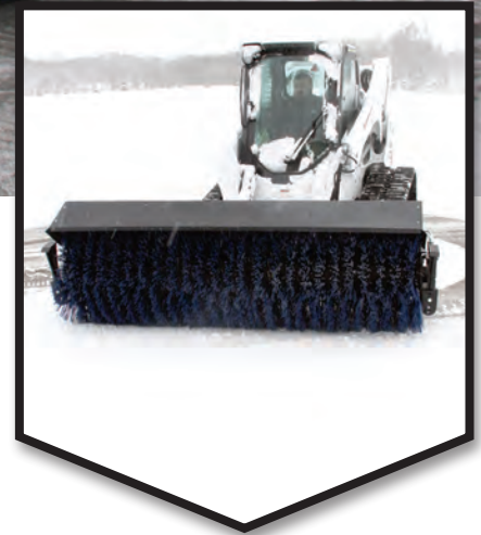
OSCILLATING DESIGN ALLOWS BROOM TO FOLLOW UNEVEN TERRAIN
