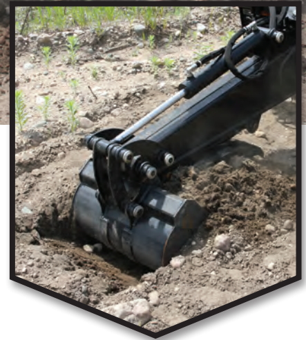
SHOWN WITH REPLACEABLE BUCKET TEETH (PIN ON) AND OPTIONAL MECHANICAL THUMB
