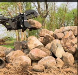
**GRAPPLE CLOSES COMPLETELY** TO SECURE LARGE AND SMALL DEBRIS
