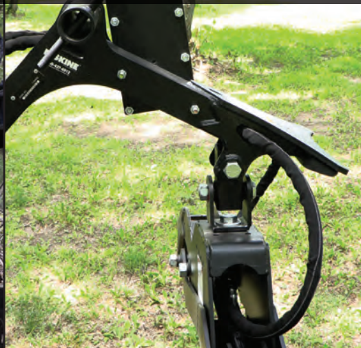
360 DEGREE MANUAL ROTATION WITH THE OPTION FOR HYDRAULIC ROTATION
