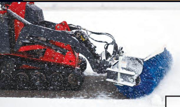
The Mini Power Angle Broom is designed for heavy-duty sweeping of dirt, snow, and other unwanted material. It quickly mounts to your mini skid steer. Featuring a 48" or 60" width and optional hydraulic angle change, this attachment is designed to go anywhere to get the job done!
