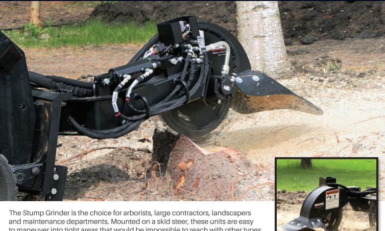
to maneuver into tight areas that would be impossible to reach with other types of machines without creating unnecessary damage to property. It features the ideal combination of maneuverability, power, durability, and simplicity.
