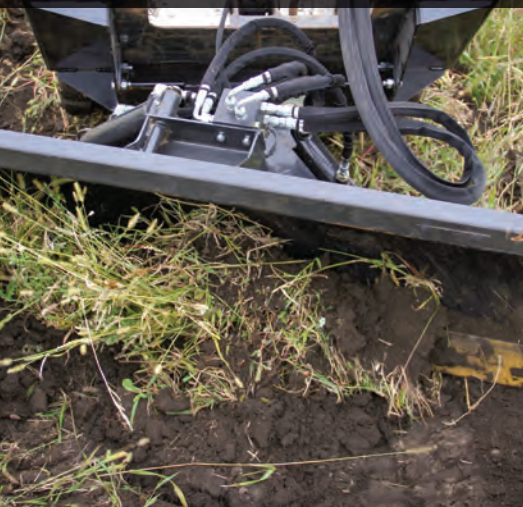
OPTIONAL HYDRAULIC ANGLING AVAILABLE FOR MANEUVERING MATERIAL
